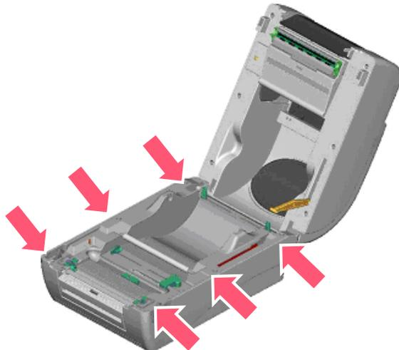
4. Upside down the printer. Remove two screws at the hinge and remove one screw at memory card cover.
